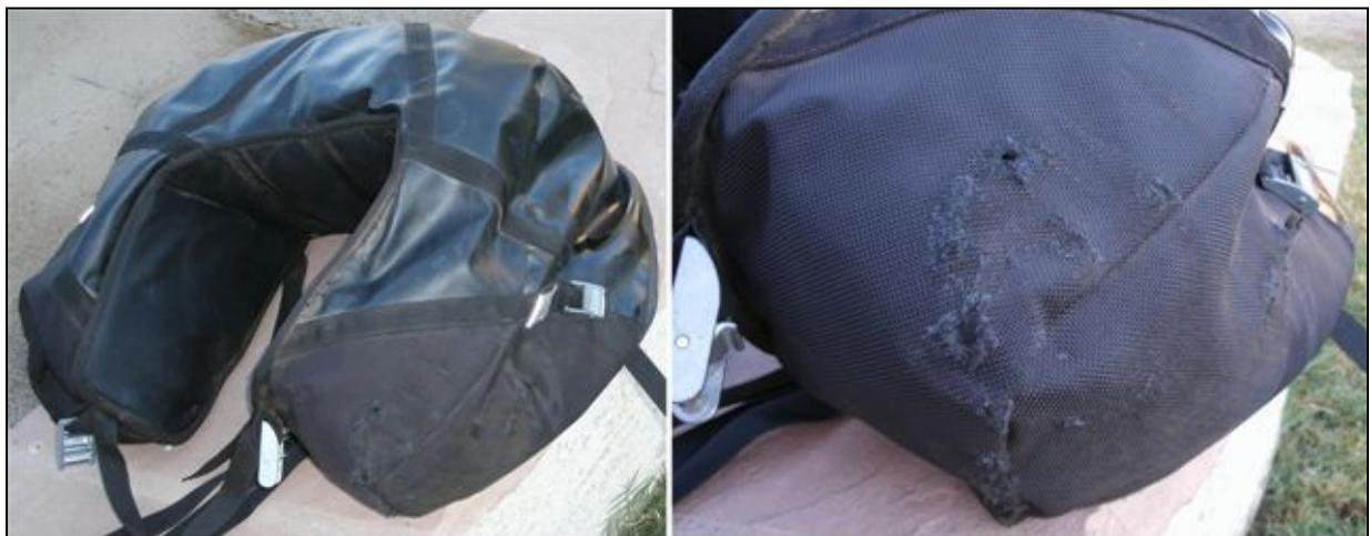
Still waterproof with minimal damage after laying it down at 45 mph.
