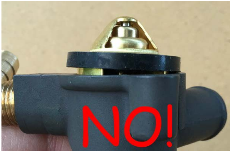
Figure 2: Improperly indexed thermostat Will not seat properly.
