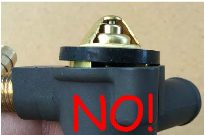
Figure 2: Improperly indexed thermostat Will not seat properly.
