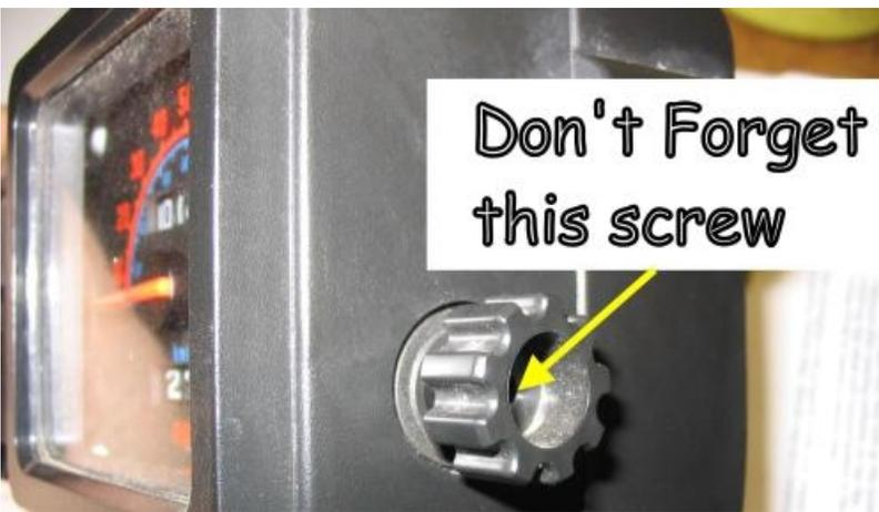
This photo shows one final screw that must be removed, down in the center of the trip odometer reset knob. Once the screw is removed, pull the knob straight out of the housing... it's a friction fit on the shaft.
