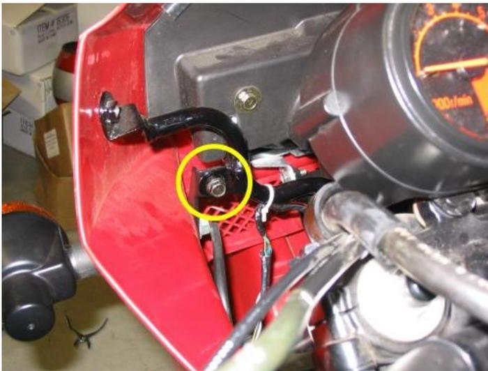
Next, you will find two bolts on the inside of the fairing with 10mm heads that need to be removed. (The left one is circled in the photo). The fairing can now be pulled forward a number of inches...
