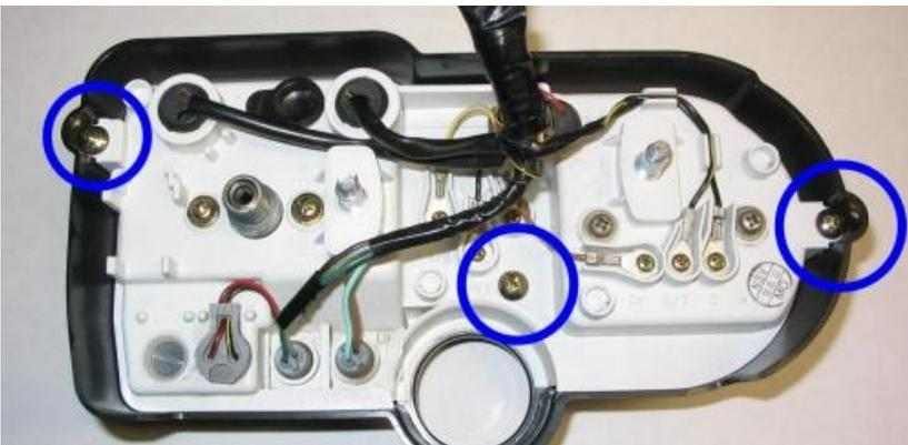
This photo shows the back of your instrument panel. Remove the three screws that have a blue circle drawn around them.
