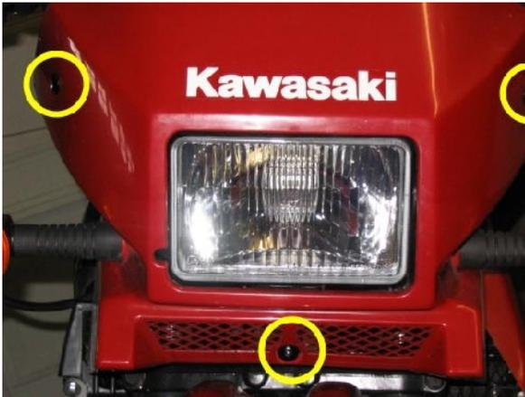
Start by removing the three screws (circled in yellow) that hold the fairing in place.
