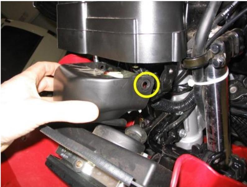
Below the instrument panel, you'll see a cover, retained by two screws. The left screw is shown in the photo. Remove both of them and set the cover aside.
