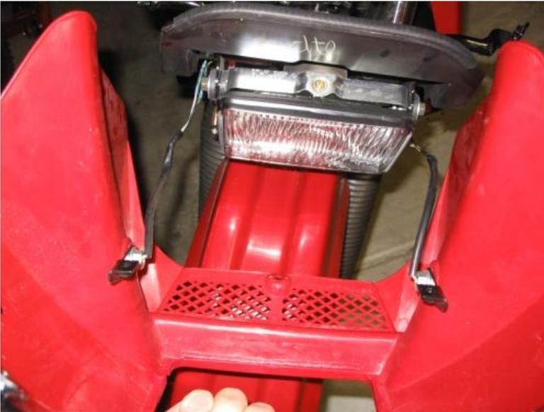
Where you'll see that only the turn signal wires are holding it as shown. Disconnect the four turn signal wires (two sets of two) and set the fairing aside.
