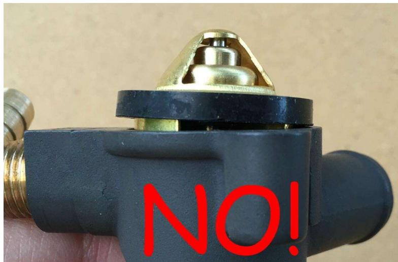
Figure 4: Improperly indexed thermostat Will not seat properly.
