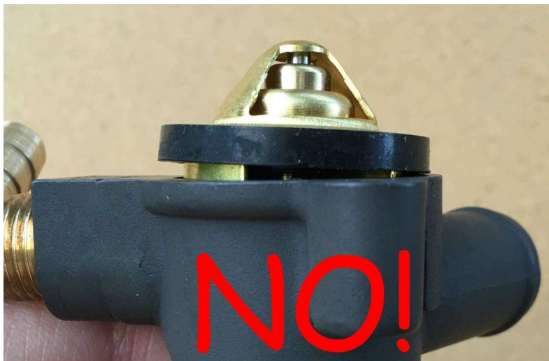
Figure 6: Improperly indexed thermostat Will not seat properly.
