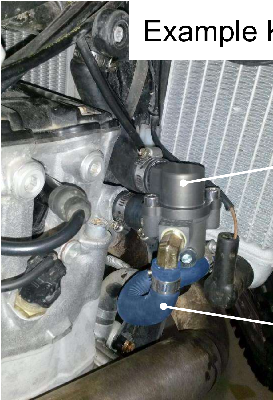
Figure 4: Installation using factory bypass hose
