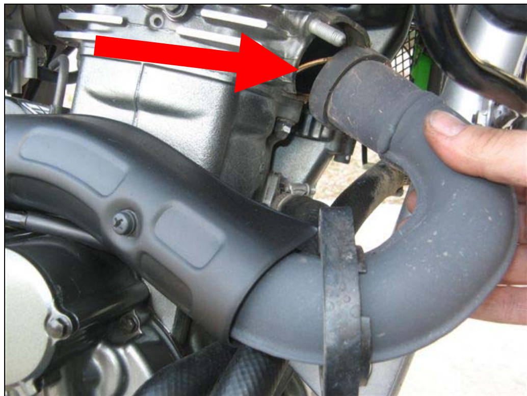
Figure 6 (Red Arrow points to copper crush washer)
