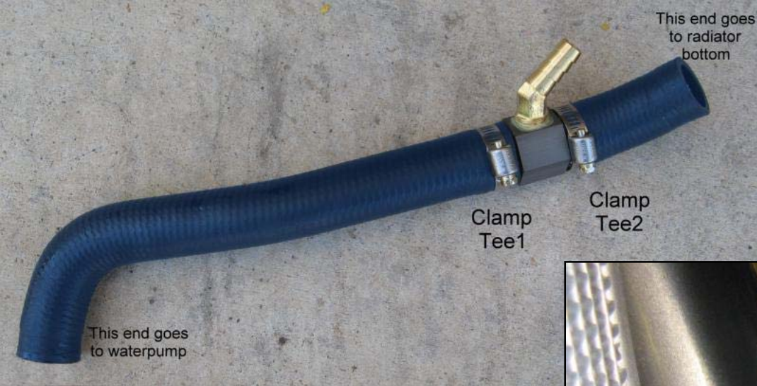
Figure 31: Tee Installed in lower hose.
