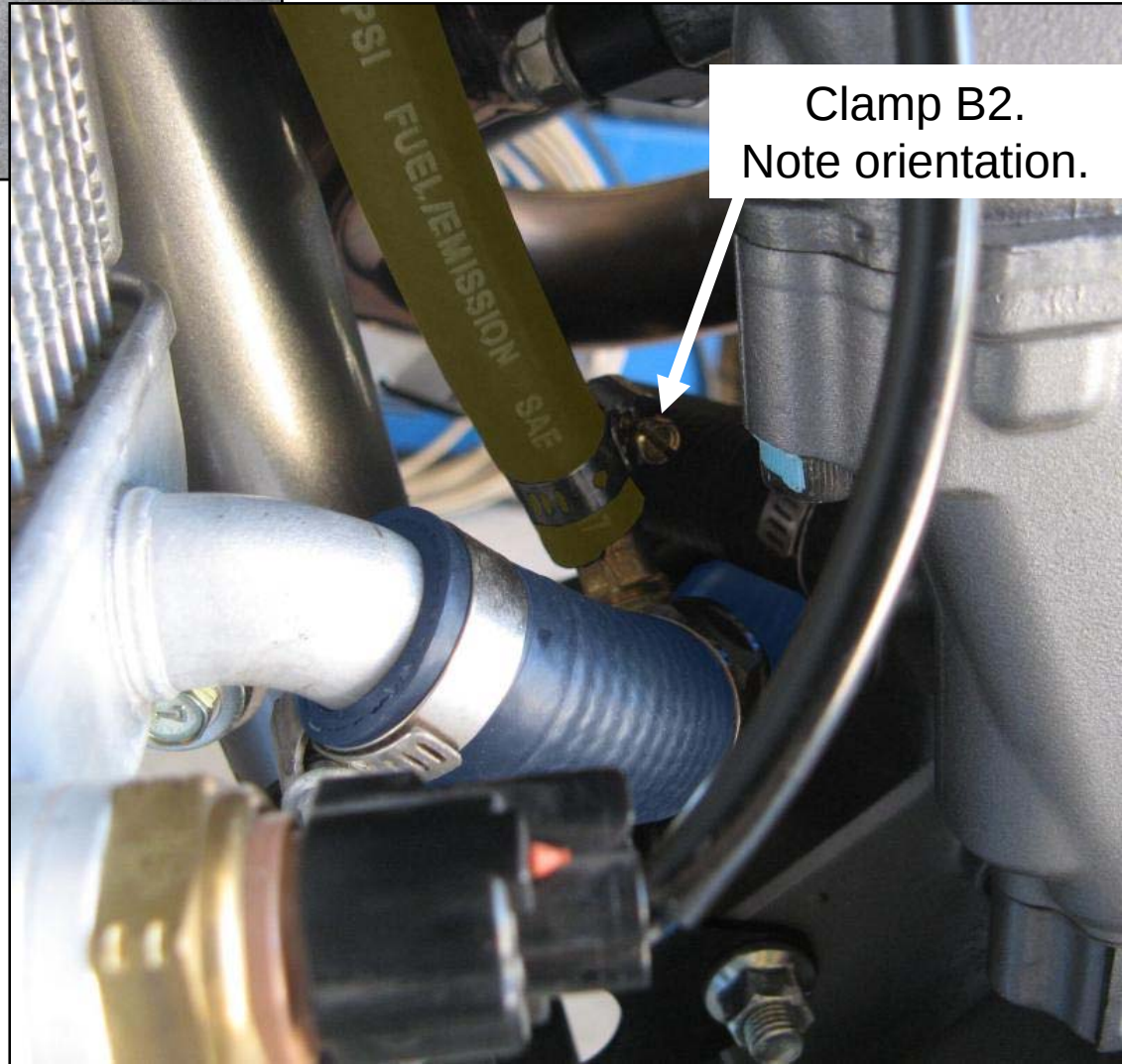
Figure 32: Details of complete installation of lower radiator hose and bypass hose connection.
