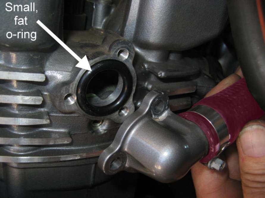
Figure 27: Attach upper hose to cylinder head with o-ring in place (see Step 15 of instructions for fastener torquing process).
