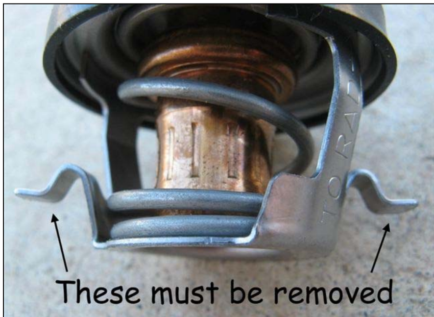
T-stat with full tabs still in place
