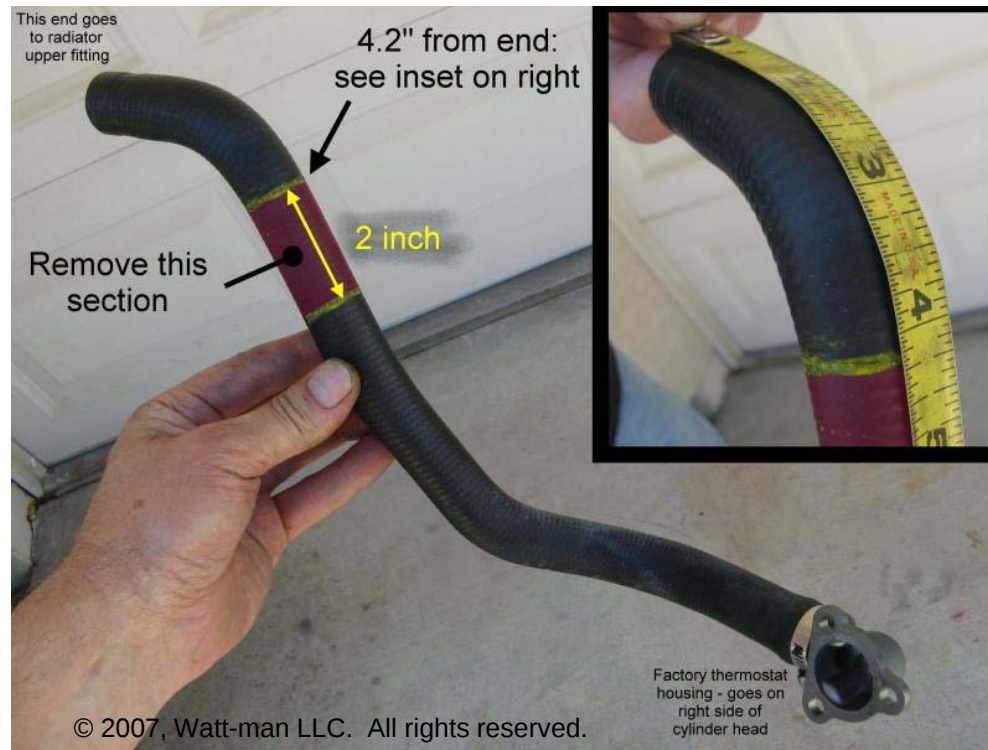
Figure 22: Remove 2 inch section from upper hose.
