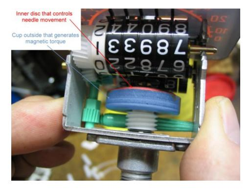
Under the odometer face is a disc that controls the needle movement (the cup outside of it generates a magnetic torque proportional to velocity and moves the inner disc). I've colored these two parts to help you visualize what I'm trying to describe. The trick here is to do this once, not over and over again as a trial-and-error project
