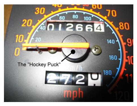
So the goal was to tweak the needle on the shaft until this same test resulted in a 30 or 31 mph reading. You'll note that the needle assembly is a black 'hockey puck' with a red/orange needle. You don't want to break off the needle, so your goal is to apply your twisting force to the hockey puck, if you will. The forces to spin the needle on the shaft were pretty high in my opinion so I was cautious, and it took a number of tries.
