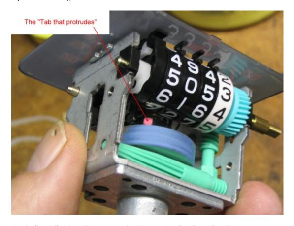
On the inner disc is a tab that protrudes. Remember that I've colored two parts here red and blue, but your parts will be silver. The tab is the easiest thing to grab on the disc, and by looking through the side (come up with the method you prefer, just be consistent!) I would center the tab at a landmark under the speedo face. While holding at this location, my daughter said it read dead on 35 mph. I did this test a few times to see if we were repeatable at getting a reading of 35, and we were.
