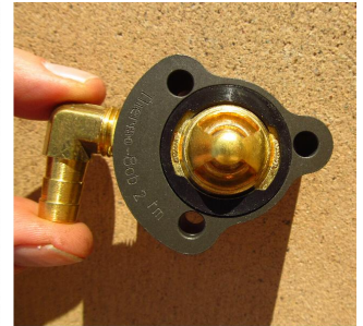
Figure 8. Install Thermo-Bob 2 thermostat in Thermo-Bob 2 Housing.
