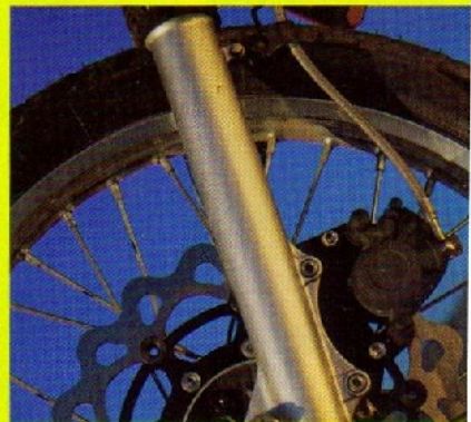
Oversized brake rotor from Galfer requires a mounting bracket that moves the stock calliper farther outboard. Stopping power is increased dramatically.
