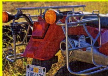
Not only does the rack support the luggage, it also keeps it from burning on the muffler, in this case an RT5 slip-on from Jardine.
