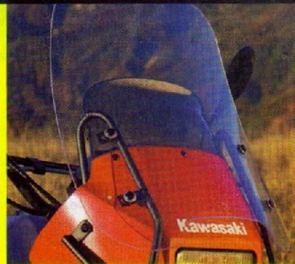
TCI Products windscreen is a bit unusual in that it mounts on top of the stocker. Of course you have the option of removing it.
