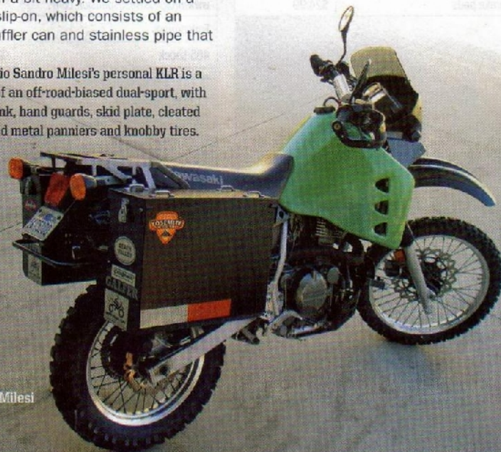
Not only does the rack support the luggage, it also keeps it from burning on the muffler, in this case an RT5 slip-on from Jardine.
