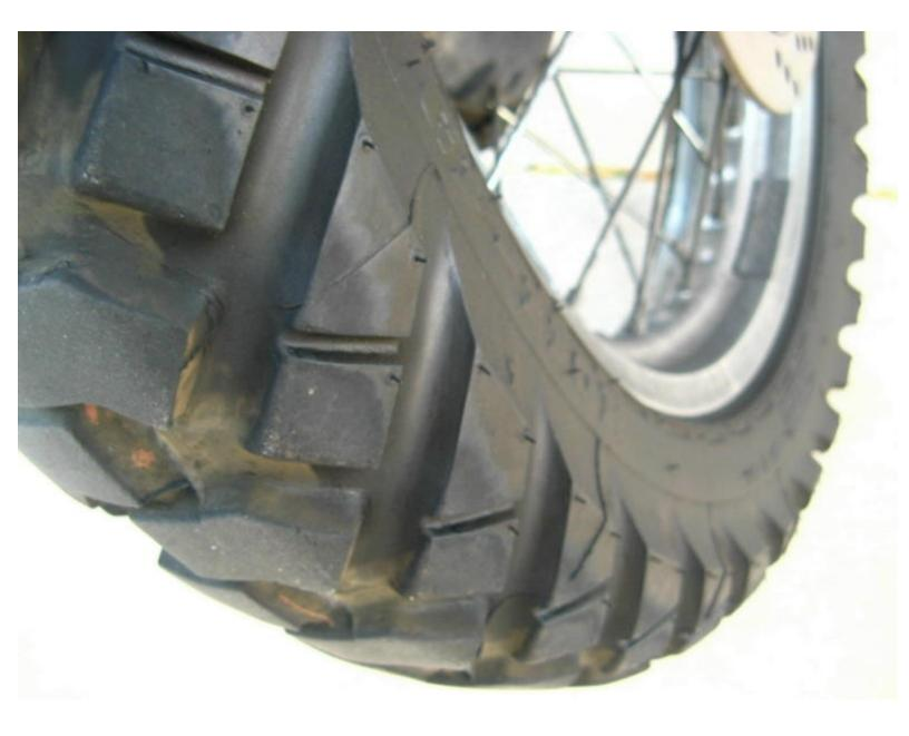
But now let's lean it way over – such as aggressive cornering on the street. See how the side knobs are built into the carcass of the tire? This way they don't flex a lot, and the tire grips well in aggressive street cornering. This tire is not squirmy on the street at all when heeled over. I've been riding which a number of street-tired KLR guys and still seem to put distance on them when in the tight stuff. They're usually not amused.
