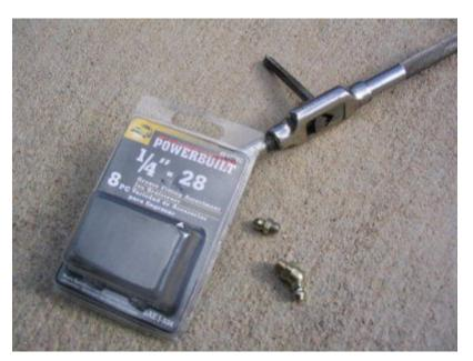
3) Zerks are available at most auto part stores. These have a convenient 1/4"-28 male thread on the ends as shown above. I was able to purchase a set of 8 for \$3. The other tools needed (other than drill bits) was a 1/4 - 28 tap, and a vise or press with a large selection of sockets. I didn't feel comfortable doing all the machining with the bearings installed, so with the method shown below I pushed the bearings out of the housings before doing any drilling.
