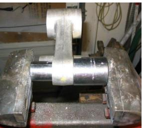
In this photo you can see how socket size choice is the key - as you tighten the vice, the left (small) socket pushes the internal bearing to the right, into the right (large) socket.
