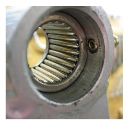
1) As referenced earlier, each of the six pivots have needle bearing(s) inside. With the grease seals out as shown above, the idea is therefore to put grease in on one side of the bearing...
