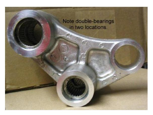
Next is the lever, using the same basic procedures. Two of the pivots are easy as they have double bearings each, so you put the zerk in the center and the two vent holes past the bearings. The third zerk fitting is tight because it's a single bearing - and hole placement must be reasonably precise. The next 5 figures (on the next page) show the details.
