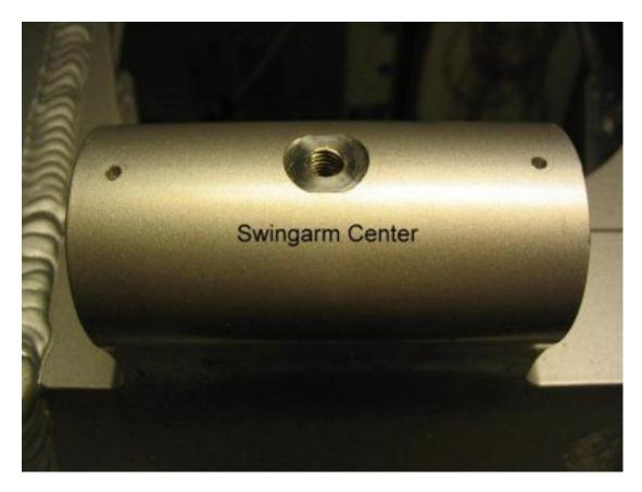
6) These two figures show details of the final location on the swingarm - actually the easiest to do as there are two bearings, one on each end. Simply place the zerk in the center, and if you want, put two vent holes in - one on the outside of each bearing. I've since installed a 45° zerk instead of the straight (shown) for easier access when installed on the bike.
