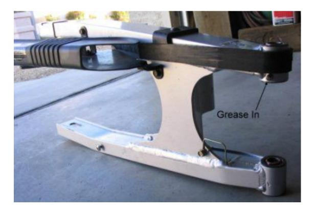
The figure above allows you to see the third swingarm zerk fitting, which is on the top of the left pivot.
