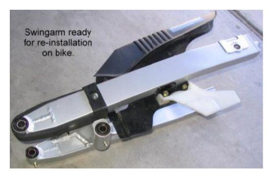
With the bearings and seals re-installed, the figure above shows the completed swingarm, ready for installation onto the bike.
