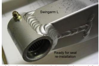
4) These four figures show details of the pivot on the left side of the swingarm. I've placed the zerk on the top right
