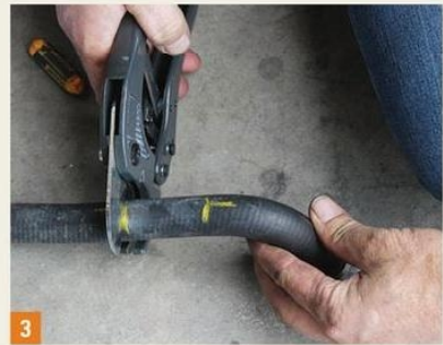
3 Clear directions tell you where to cut the hoses to place the new parts in the system and we've marked them before cutting.
