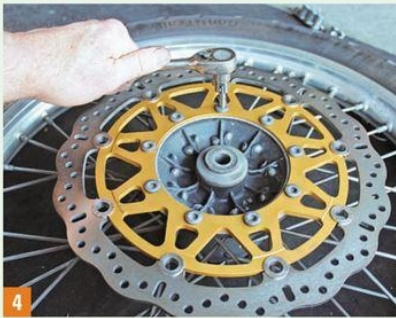
4 The new disc is installed with the old bolts. Be sure to use Loctite on the bolt threads to prevent any loosening over time.
