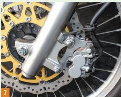
7 The Eagle caliper adapter installed. Note how the brake hose routing clip now pulls on the stock brake line, making it too short.
