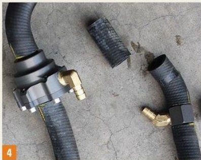
4 This close-up shows the new Thermo-Bob billet aluminum thermostat housing and brass return line fitting installed.
