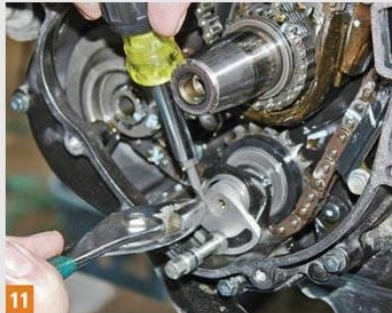
11 With pliers and a screwdriver for assistance, the torsion spring is hooked over the end of the slot in the new doohickey.
