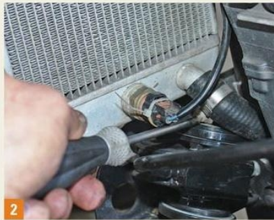
2 The return hose is a little more difficult to access but not terribly. Of course, the coolant is drained beforehand.
