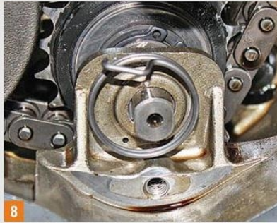
8 Here, the new torsion spring is located in position. A \frac{1}{16} " hole has been drilled to accept the stationary end of the spring.
