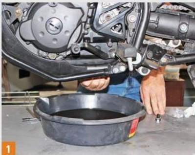
1 Tackling the doohickey begins with draining the oil, removing the skid plate and getting the shift lever out of the way.
