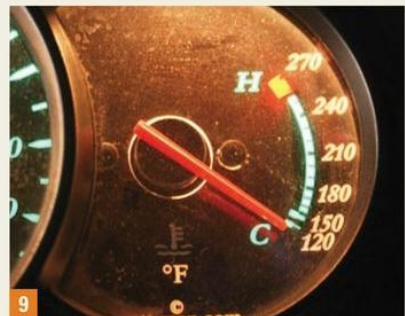
9 With the gauge reassembled, you can see how the face looks when illuminated. The numbers are claimed accurate within 2°-4°.
