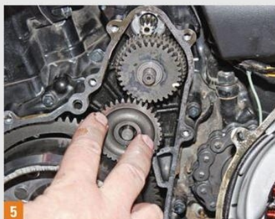
5 The intermediate gears must also be removed. Note their exact orientations so you can easily replace in the same position.
