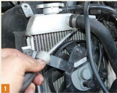
1 The Thermo-Bob installation is straightforward, and only the radiator's inlet (shown) and return hoses need to be removed.
