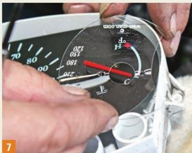
7 To accurately check on the changes with the Thermo-Bob installed, we added a calibrated face to the dashboard's temp gauge.
