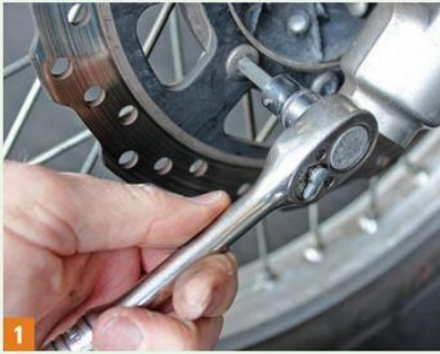
1 Installing the EBC disc kit starts with wheel removal. You'll also find it helpful to loosen the disc mounting bolts beforehand.
