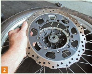
2 With the wheel off, the stock disc can be removed. Note that the old disc is fixed, not floating, which also reduces brake feel.
