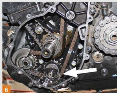
6 With everything out of the way, the doohickey itself is visible at the bottom center of the engine, tensioning the lower chain.
