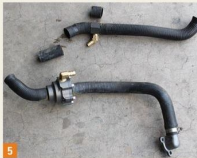
5 Above shows the full length of the hoses and the positions of the new parts as they fit into the system.
