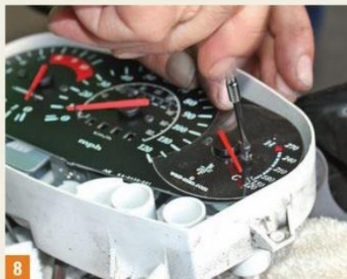
8 While the standard gauge gave an indeterminate scale from hot to cold, the new face plate adds accurate numbers to the range.
