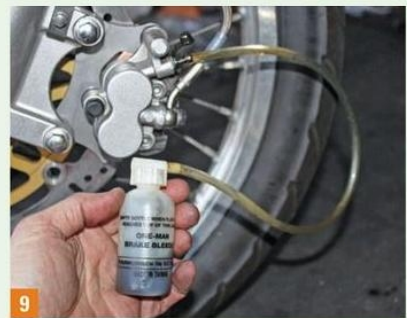
9 We found conventional bleeding of the dry brake hose too tedious (above), so we used a Mityvac pump to simplify this operation.
