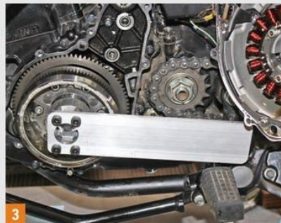
3 To remove the rotor's holding bolt, you must use a holding tool. Use a fresh bolt for refitting as it requires 130–144 lb.-ft. of torque.
