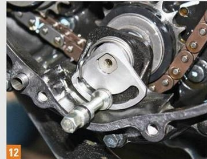
12 With the adjusting bolt in position, you can visualize how it works, loosened at TDC on the compression stroke and retightened.
