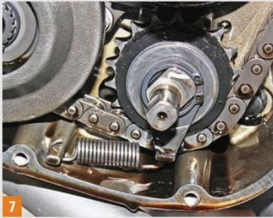
7 Close-up of the doohickey shows the stock unstretched coil spring which is meant to keep the chain tight, but doesn't.
