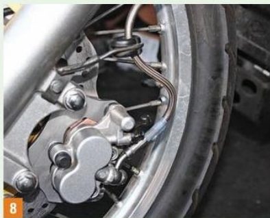
8 With the longer Russell braided brake line, the bend is no longer a problem. The braided line expands less, for a better lever feel.
