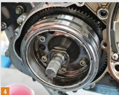
4 Because it's tightly mounted on a tapered shaft, the rotor requires a puller to remove, here shown in position.
