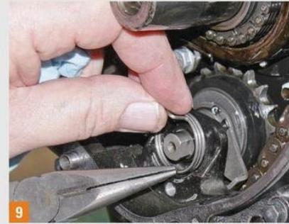
9 The round torsion spring must be fitted into the new hole before securing the other end to the doohickey lever.
