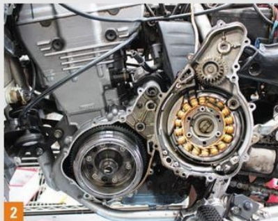
2 The outer cover isn't particularly hard to remove but the magnets make it harder than you'd figure after the 10 bolts are removed.
