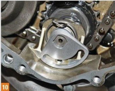
10 The new stainless steel doohickey in position over the squared shaft, ready to last forever and keep the chain tight.
