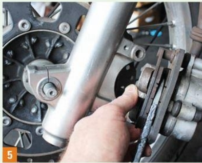
5 Use a screwdriver or tire iron to retract the caliper pistons before installing the new brake pads, so they allow room for the disc.
