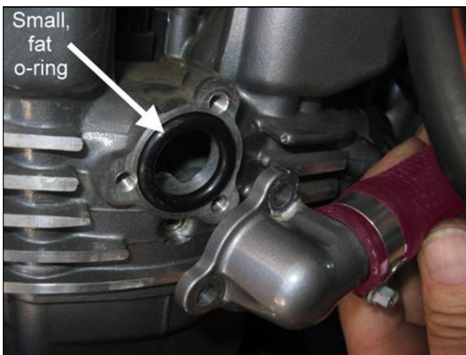
Figure 13: Attach upper hose to cylinder head with o-ring in place (see Step 15 of instructions for fastener torquing process).
