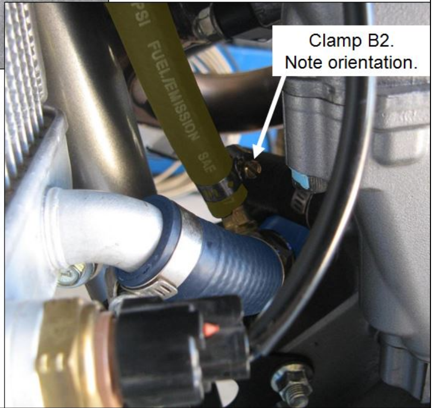
Figure 18: Details of complete installation of lower radiator hose and bypass hose connection.
