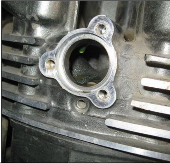
Figure 7: Remove factory thermostat and gasket.
