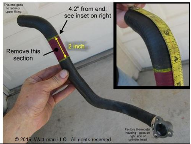
Figure 8: Remove 2 inch section from upper hose.
