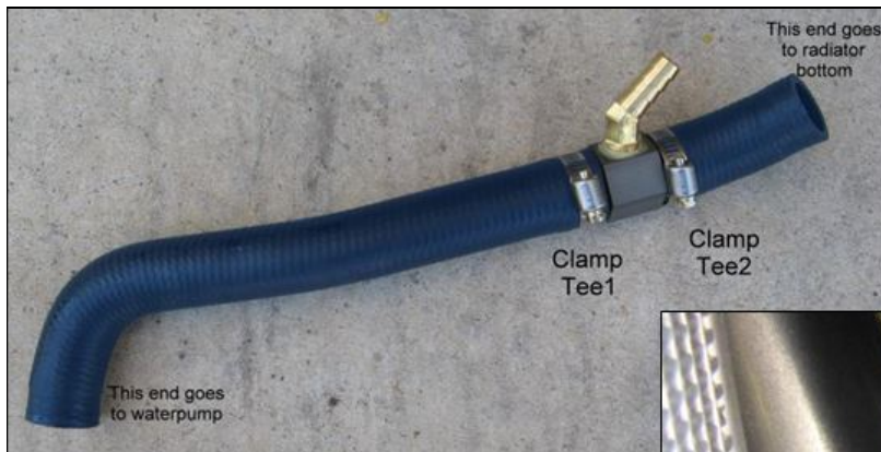
Figure 17: Tee Installed in lower hose.
