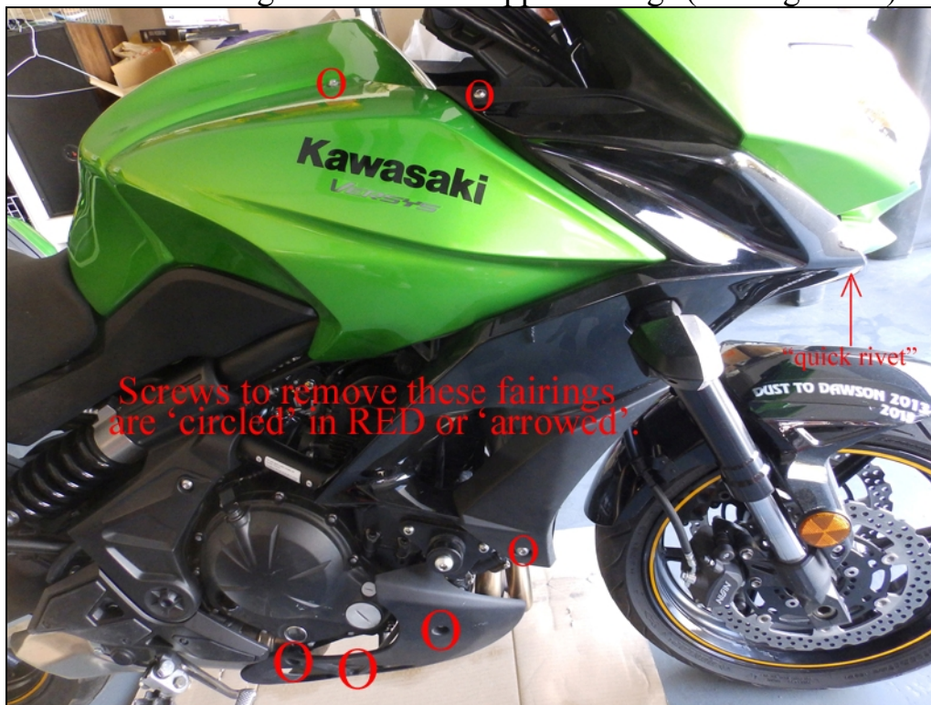
Figure 1. Screws that retain plastic bodywork.
