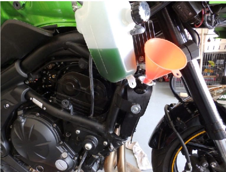
Figure 14. Time to refill the cooling system.
