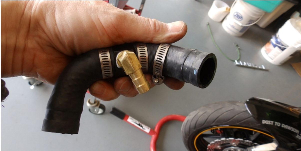
Figure 10. Bypass Tee Installed in left-side Radiator Hose.
