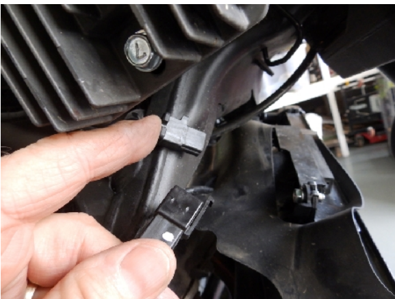
Figure 7. Cooling Fan Harness Plug.
