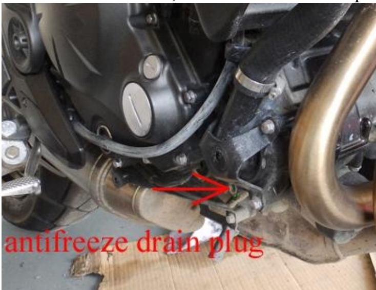
Figure 3. Coolant system drain plug is in the bottom of the coolant pump housing.
