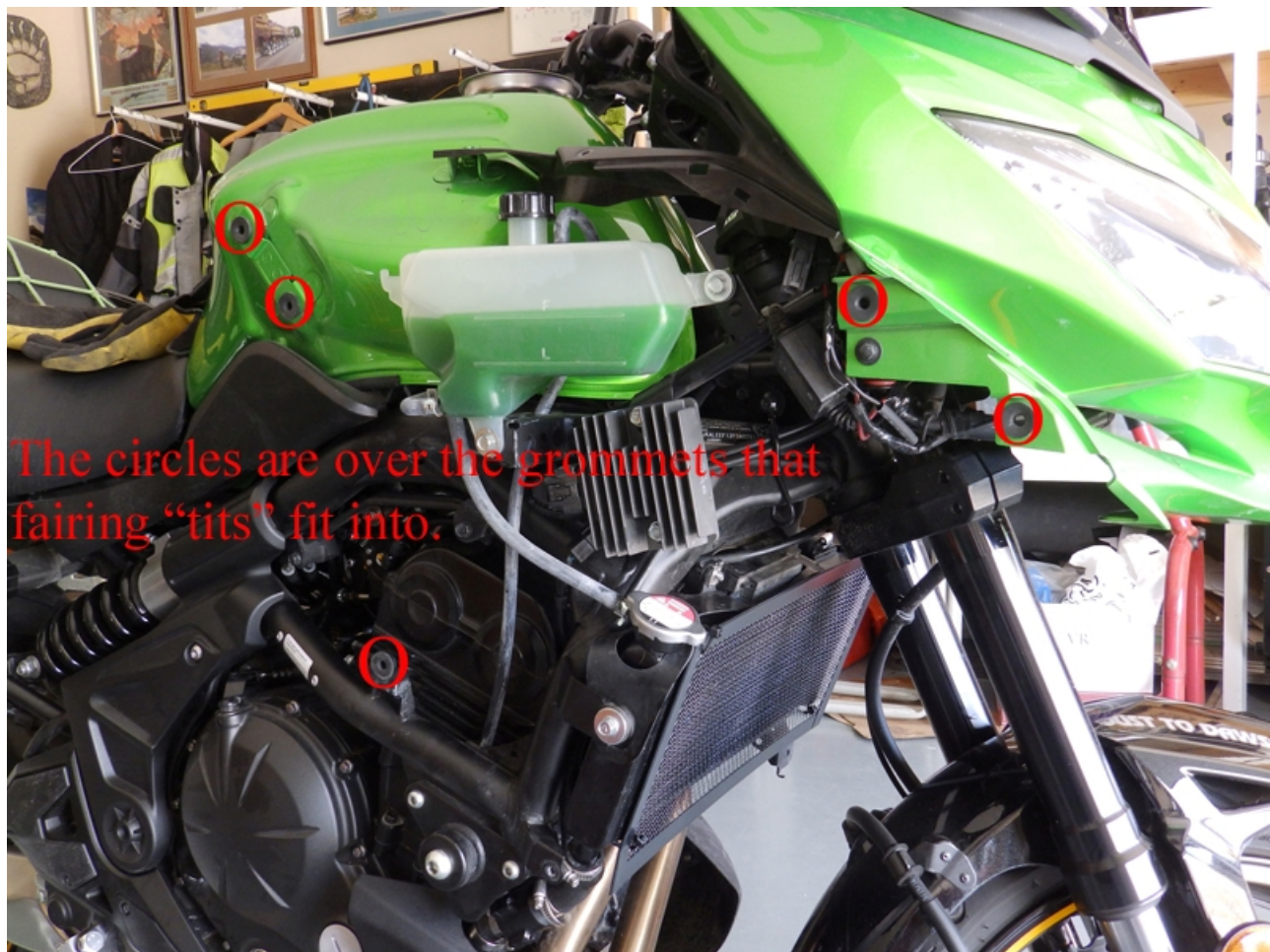
Figure 15. Five grommet locations for engagement of fairing protrusions.
