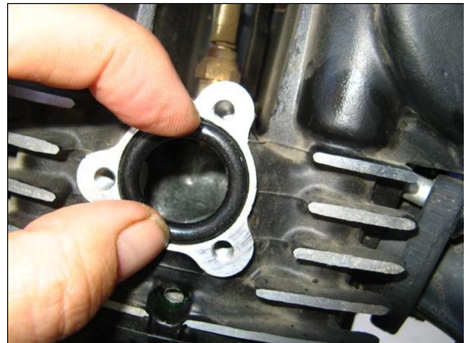
Figure 6. Place small, fat o-ring in place.
