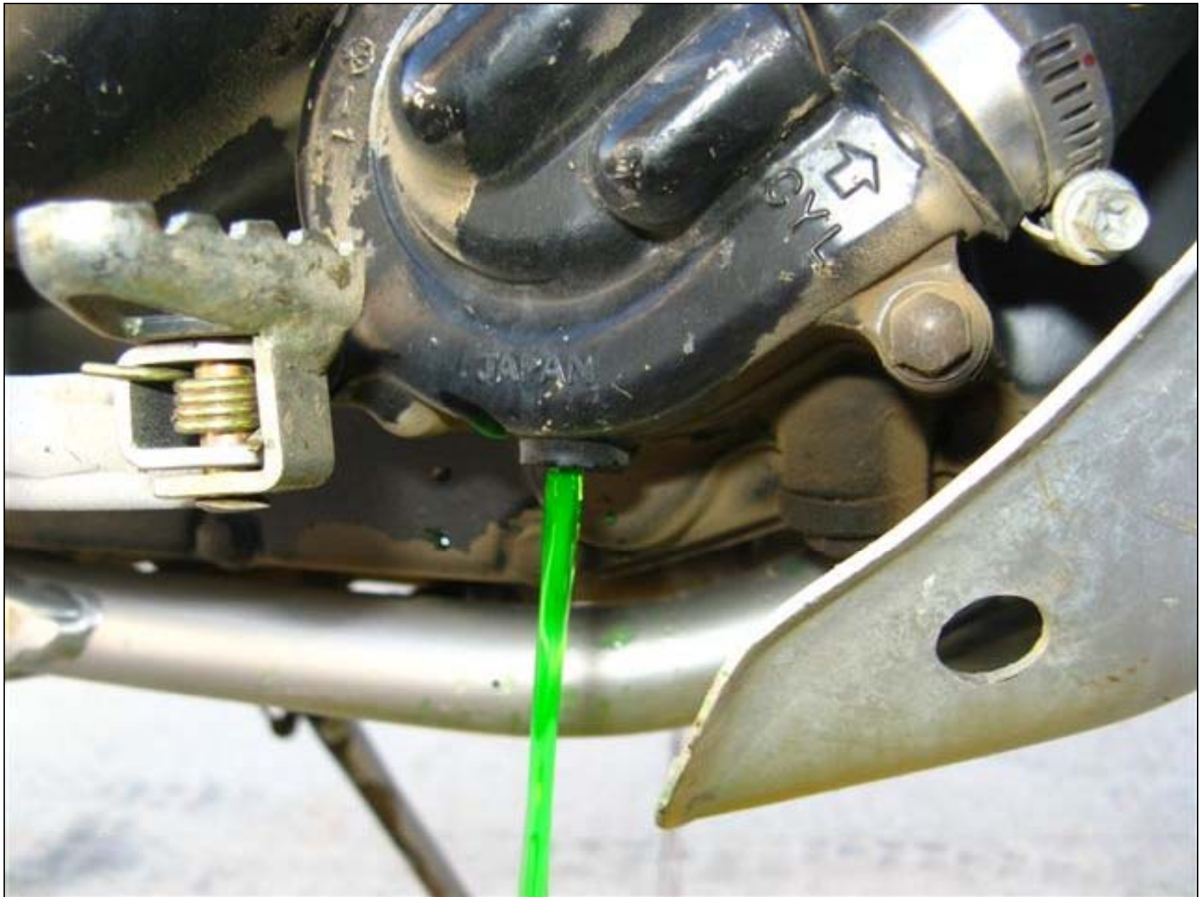
Figure 2. Drain coolant by removing drain plug at bottom of coolant pump.
