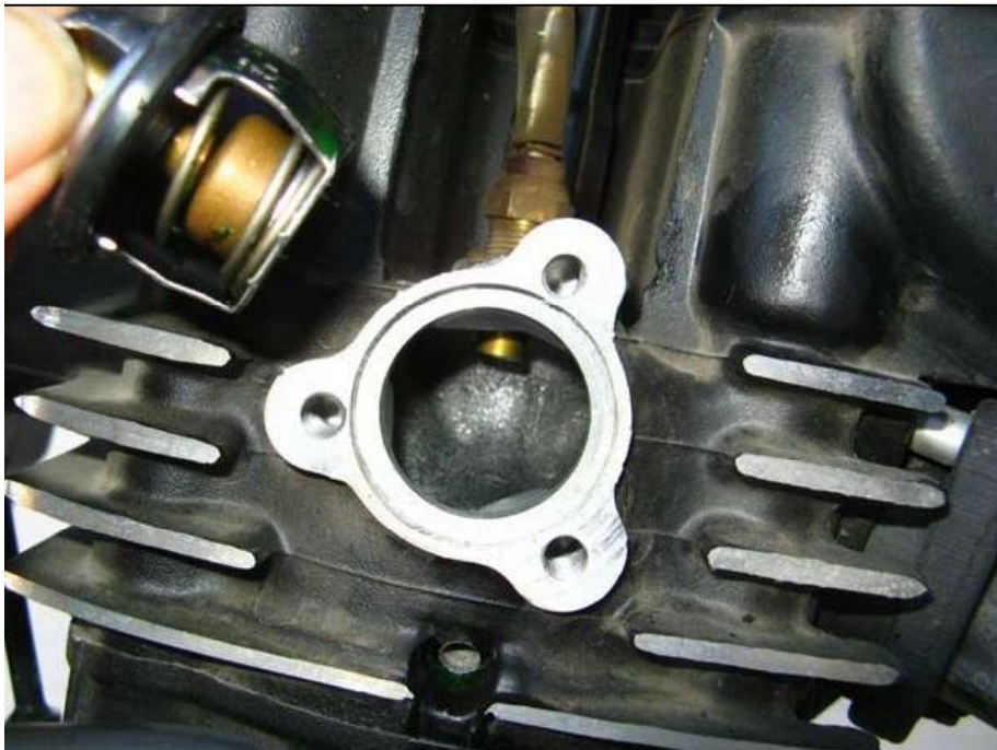
Figure 5. Remove original thermostat.
