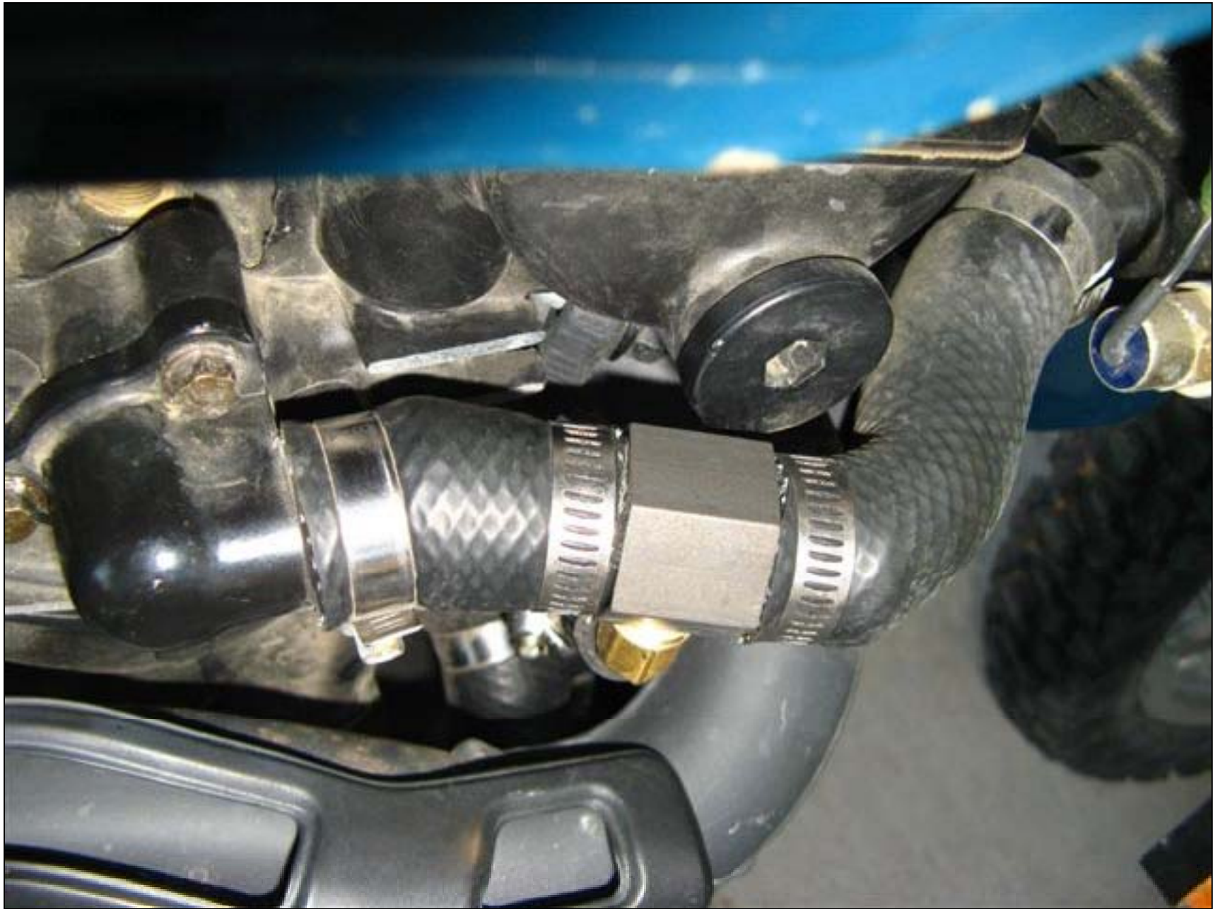
Figure 23. Tee placement in upper hose.
