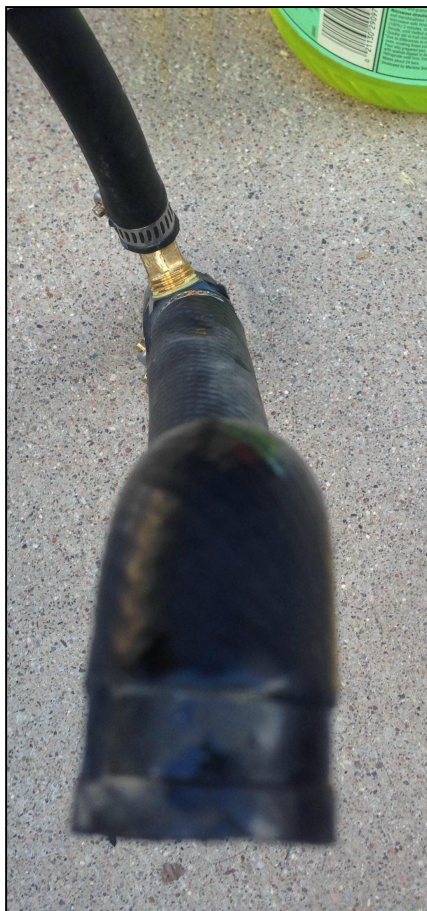
Figure 12. Orientation of barb on bypass tee.
