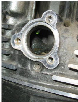
Figure 7. Remove Original Thermostat.
