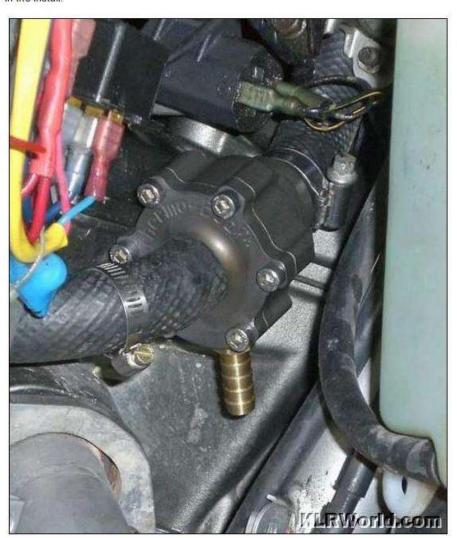
Now, specific measurements are given in the instructions as to where to cut the radiator return hose for the bypass "t" fitting. Simply measure and cut, install the bypass "T" and the clamps, and before tightening the clamps, you'll want to "aim" the thermostat housing bypass fitting and the bypass "t" fitting at each other. It makes for a cleaner install. Then you can tighten the clamps.
