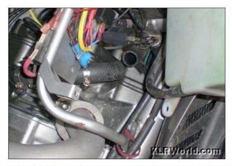
The device is actually a little wider than the 1/4" inch I left for it, but the extra hose helps to hold it away from the cylinder head. You can alter yours as needed, but start small, you can't add hose once you've cut it.
