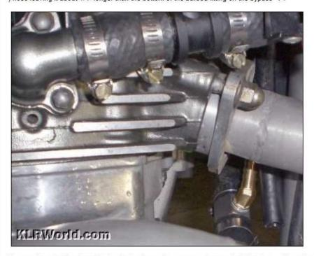
Not much to it after that. Check all the hose clamps, use the supplied Zip-tie to adjust the position of the thermostat housing as needed ( I didn't need it ), fill with coolant per the instructions, reassemble, and ride.
