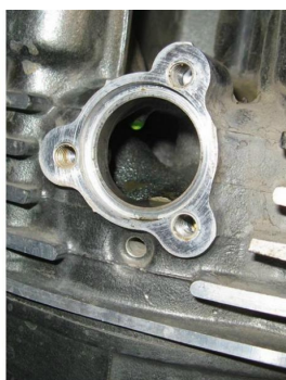
Figure 7. Remove Original Thermostat.
