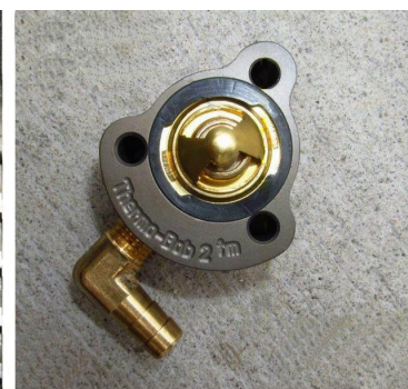
Figure 8. Install Thermo-Bob 2 thermostat in Thermo-Bob 2 Housing.
