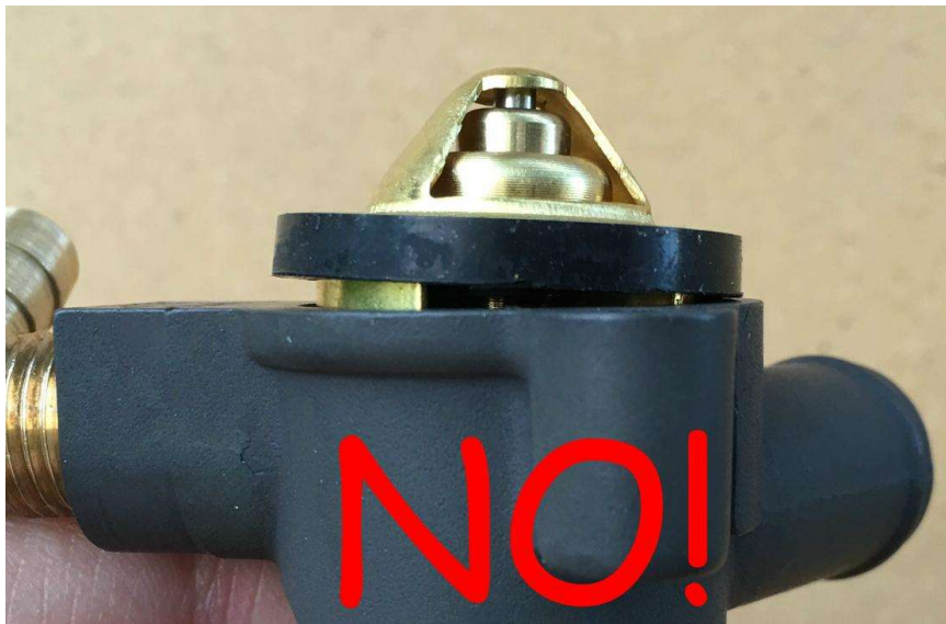
Figure 2: Improperly indexed thermostat Will not seat properly.
